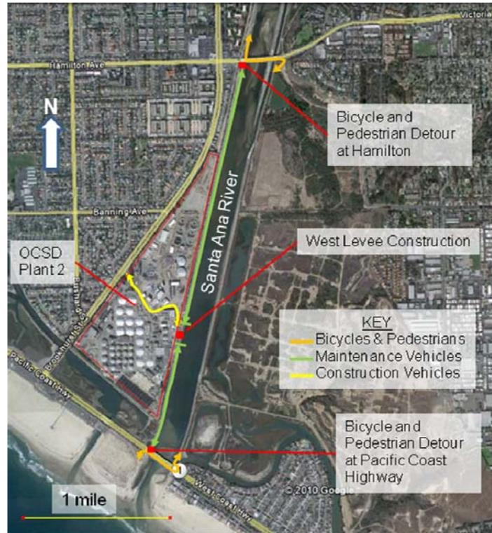
**Figure 7: Traffic Detour Pattern for Construction on the West Levee**
